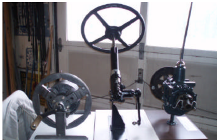
Cutaway assemblies of a Model A transmission, Steering column and a Model T transmission Items from past seminars
